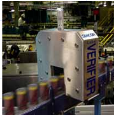
Single file conveyor installation
